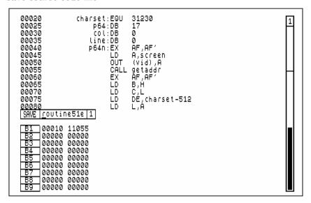
The illustration shows the screen when the **+s** command is entered. The SAVE information is displayed at the bottom left of the screen.
