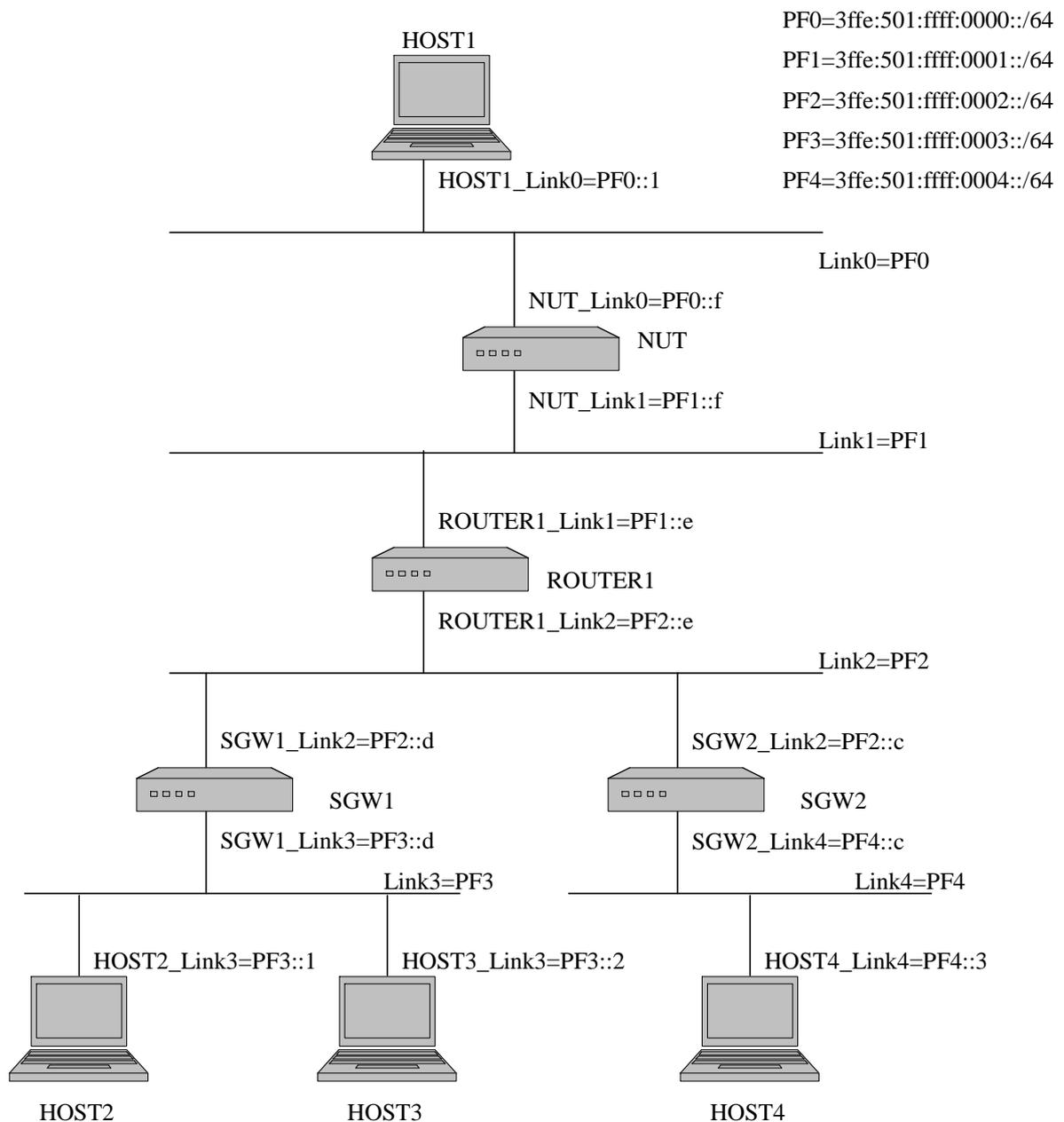
Fig. 4 Topology for SGW: Tunnel mode with SGW
