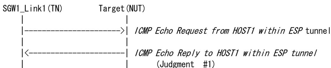
1. SGW1 sends "ICMP Echo Request from HOST1 within ESP tunnel"
