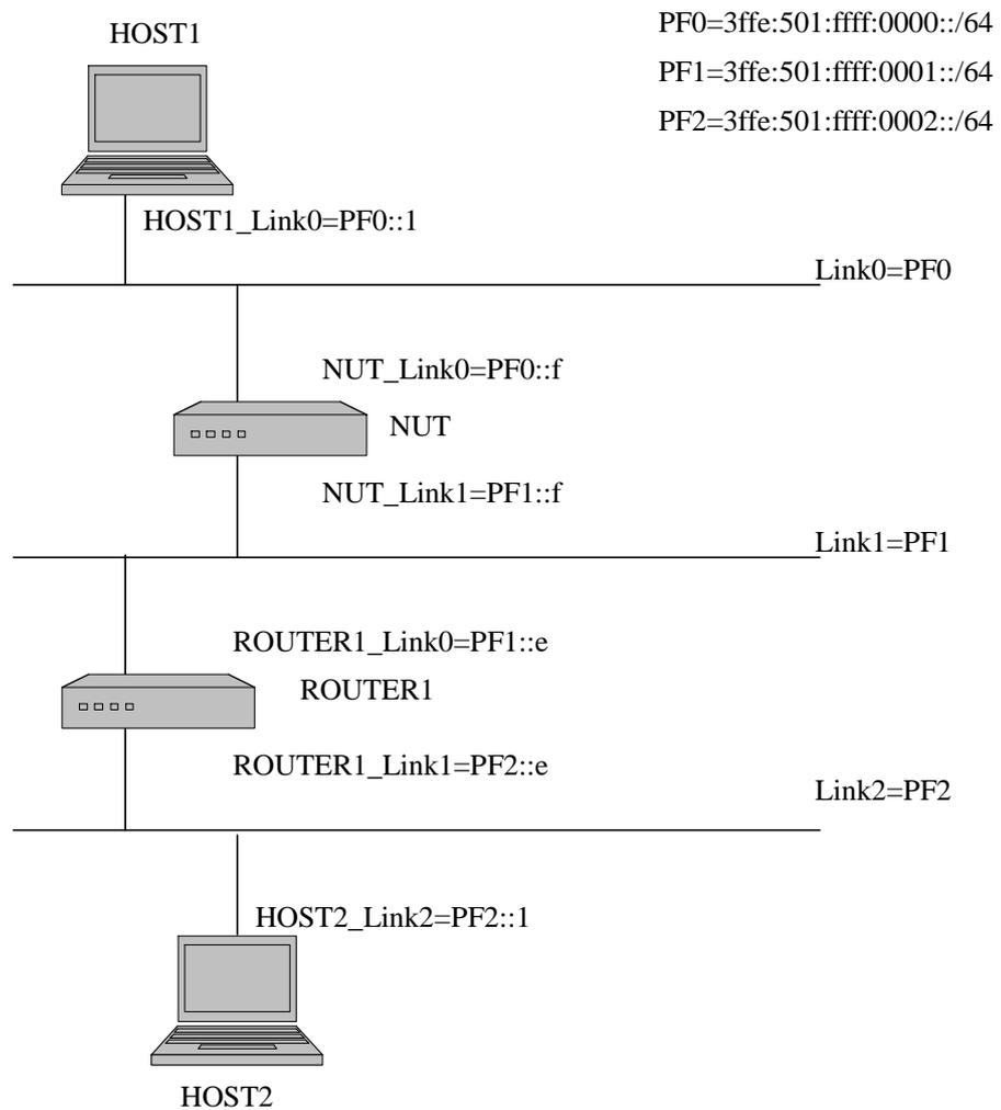
Fig. 3 Topology for SGW: Tunnel mode with End-Node
