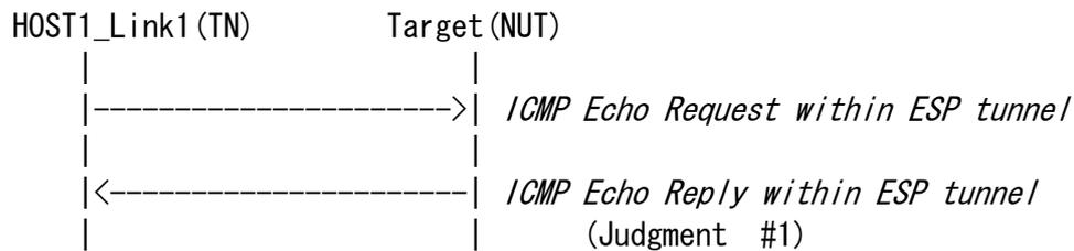
1. HOST1 sends "*ICMP Echo Request with ESP tunnel*"
