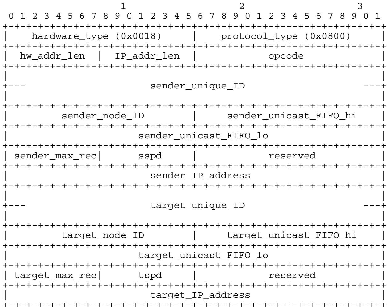
Figure 5 - ARP request/response format
